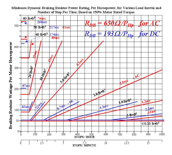
The above graph is for **480VAC** drives. It allows the power dissipation rating of dynamic braking resistors to be determined if the total mechanical inertia at the motor and the number of stops per unit time are known. The graph provides the wattage required per horsepower of motor load with a braking level of **150%** of rated toque and
